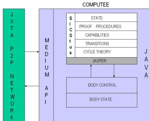
Figure 2: Implementation architecture of a PROSOCS computee (SOCS-iC)
