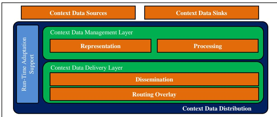
Fig. 1. Context data distribution system logical architecture
