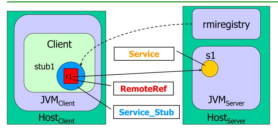
The **Client** uses the **RMI Server** implemented by the **Service** class exploiting the reference to the local stub *stub1* (instance of the **Service\_Stub** class provided to the client by the registry) **Service\_Stub** contains a **RemoteRef** (*r1*) that allows the RRL to reach the server
